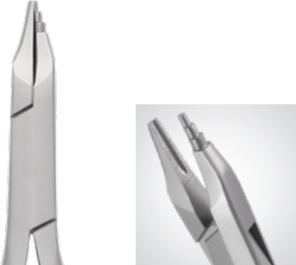
3000/95 Tweed – Short ø max 0,5 mm / .020" mm 135 Designed to form precise omega loops. Short grooved beak internally serrated. Short type.
