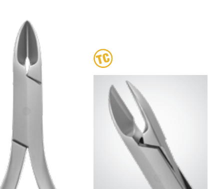
3000/89 TC ø max 0,3 mm / .012" mm 120 Delicate cutter, specially designed for the removal of soft stainless steel ligatures.
