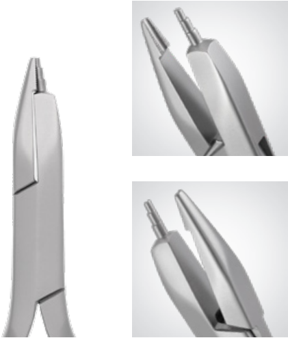
3000/97 Tweed – O'Brein ø max 0,7 mm / .028" mm 140 Graduated cone to form precise omega and closing loops. Micro serrated beaks to prevent wire slippage.
